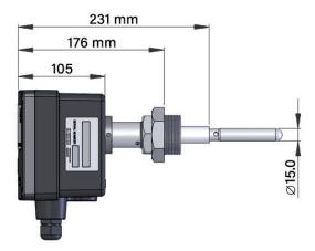
PROBE ROD LENGTH 300mm | 600mm | 1000mm
